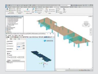
+ Automatic generation of 3D reinforcement for beams, columns, walls and slabs using results from analysis and design (also for SOFiSTiK design results of version 2016).
