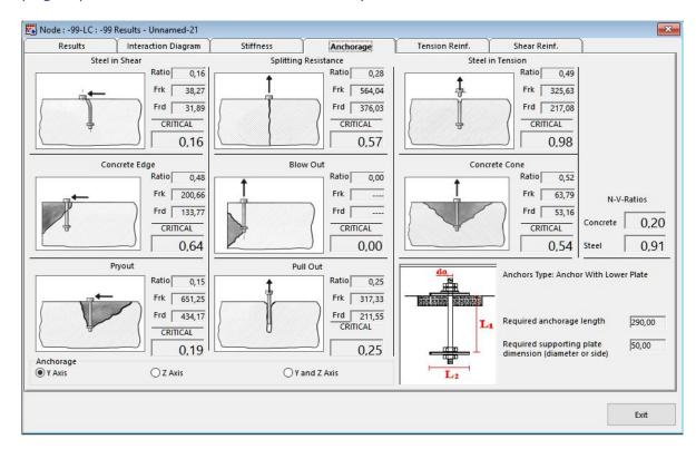
These checks are very hard to nearly impossible to be met without using any supplementary reinforcements. In this new version of the program, the user is able to calculate the additional tension or shear reinforcement bars in order to not allow concrete crack lines to be formed.
